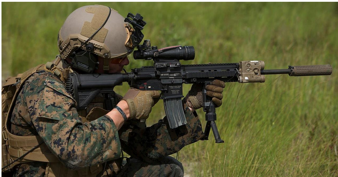
An Infantry Marine conducts live fire training aboard CLNC. Could we lighten this rifle and make it more portable? We're back to M16A4 overall lengths with the addition of a suppressor and M1 Service Rifle weights with all the attached enablers. Photo: II MEF COMSTRAT
