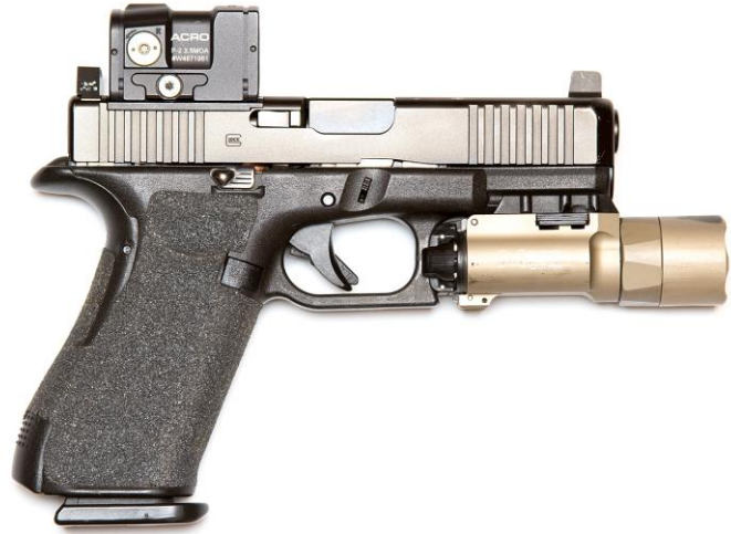
(Above): My General Purpose sidearm is a GLOCK 45 MOS (Modular Optic System) 9x19mm pistol with Aimpoint ACRO P-2, Trijicon suppressor height sights, and a Surefire X300U-A Weapon Mounted Light (WML). I attach the WML when appropriate. The long floorplate 17-rd. magazines are “borrowed” from my GLOCK 47 (US CBP contract) for removal when iced and wearing gloves.
