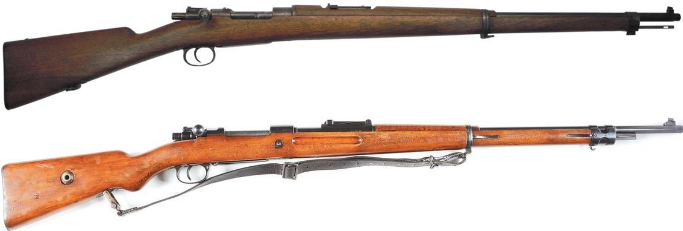
(Top): A Spanish Mauser 1893 rifle in 7x57mm Mauser. (Bottom): A German Mauser Gewehr 98 7.92x57mm Mauser. Photos: Open sources.
