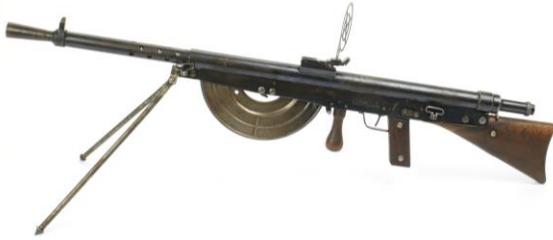
The infamous WWI-era French Chauchat “machine rifle” which was often used by Marines in the manner of a light machine gun instead of as an automatic rifle. This 20-pound weapon had numerous flaws and suffered a poor reputation, however deserved. Photos: Open source.
