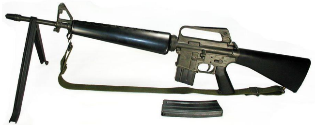
Remember this? M16A1 with bipod in the "automatic rifle" configuration. Photo: Open source.
