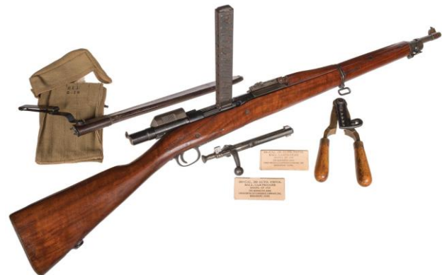
(Above): Components of the Pederson Device- Bolt group, carrying case, pouches, magazines, spanner wrench. (Below): Springfield M1903 rifle with Pederson Device installed into receiver. Note boxes of .30-18 (7.65x20mm) ammunition. Photos: Open sources.
