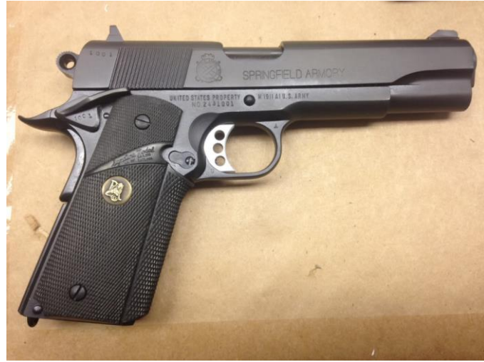
(Above): A USMC MEU(SOC) .45 ACP pistol, manufactured from select M1911A1 frames with after market parts. These pistols were employed, for a time, by the Force Reconnaissance detachment assigned to USMC MEUs. Photo: USMC.
