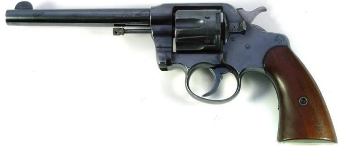
(Above): The Colt M1892 New Army and Navy, 6-shot double action revolver in .38 Long Colt.
