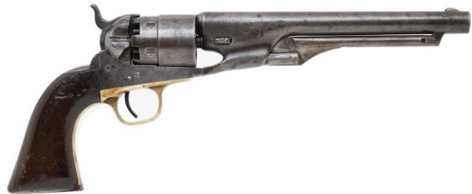
(Above): The .44 caliber black powder, percussion cap Colt M1860 Army revolver saw extensive use during and after the American Civil War.
