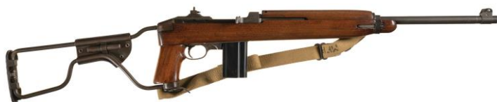
(Above): An Inland M1A1 "Paratrooper" Carbine with a folding stock for airborne operations.
